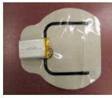
Working prototype of the Modular Stimulation System for transcutaneous electrotherapy.
