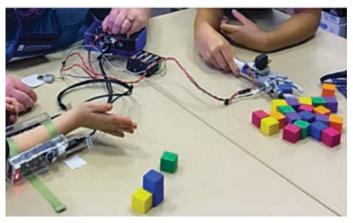
Picking up blocks using the EMG-powered robotic claw
