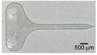
Nanocomposite-based probe with a micromolded, microfluidic channel running through it
