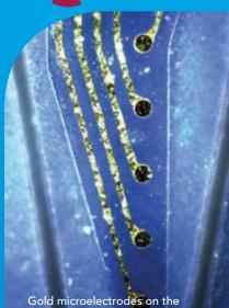
Gold microelectrodes on the polymer nanocomposite substrate
