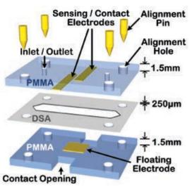
Fabrication drawing of the ClotChip sensor
